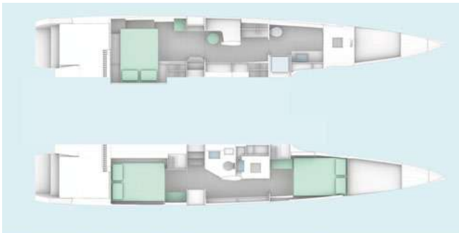
Windelo 50 - hulls plan for nacelle with U-shaped galley 1 master cabin, 1 separated WC and 1 forward head 2 guest cabins, 1 separated WC and 1 central head
