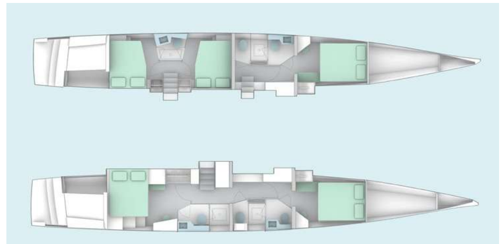
Windelo 62 – Proposed 5-cabin hull layout compatible with J-shaped galley: 1 owner's suite, 1 guest suite, 1 separate toilet 1 guest suite, 2 double cabins with shared bathroom and central toilet, 1 separate toilet
